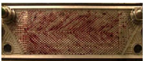
b - Jam fouling after water flow
